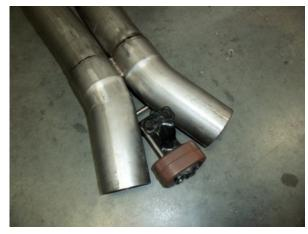
• Install the left and right x-pipe extensions with the single bolt clamps on the notched end of the extensions into the position shown. Tighten the band clamps enough to hold the extensions into place **but still allowing the extensions and band clamps to be rotated** into final position before completely tightening.
