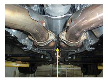
Unbolt factory catalytic converters from the manifolds and where they attach to middle part of the exhaust and remove them on both sides.
