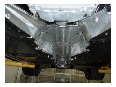
Unhook the rear 02 sensor harness on both sides from the factory retainer clip so they will reach the rear 02 sensors when they are reinstalled at a later step. Also plug in the supplied rear 02 sensor cable extensions.
