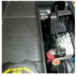
Loosen the electrical connectors from the lower fuse box tray and slide them out so the tray can be removed and remove the tray.
