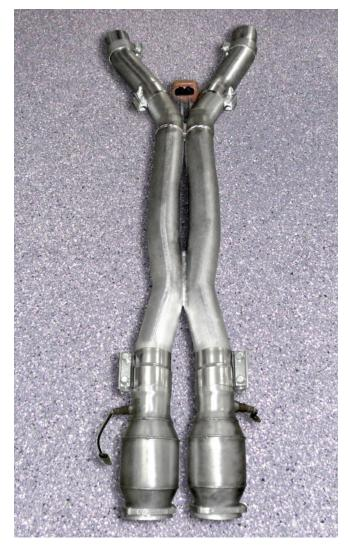
• Support the center of the x-pipe and slide the x-pipe extensions into the factory connection of the exhaust. Raise the x-pipe until the converters level with the donut gaskets on the headers.
