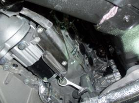
Unbolt the rear of the center of the exhaust at the single bolt clamps. Slide it toward the front of the car to remove it from the rubber hanger mount and the single bolt clamp connection.
