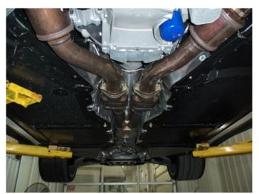
Remove the left and right aluminum cross braces.
