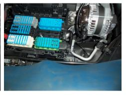
• Unhook the power terminals from the lower fuse box tray.
