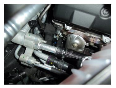
Remove the covers over the valve covers on both sides of the engine. Remove the plug wires and spark plugs on both sides.
